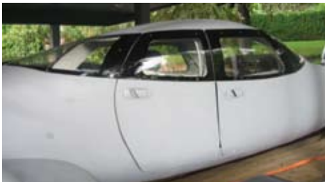
Initial fabrication and prototype construction has been carried out using hand-crafted fiberglass
