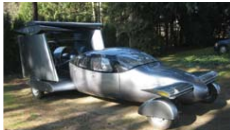
The wings, canards and rear wheel fixtures are able to move, then lock into flying or driving mode
